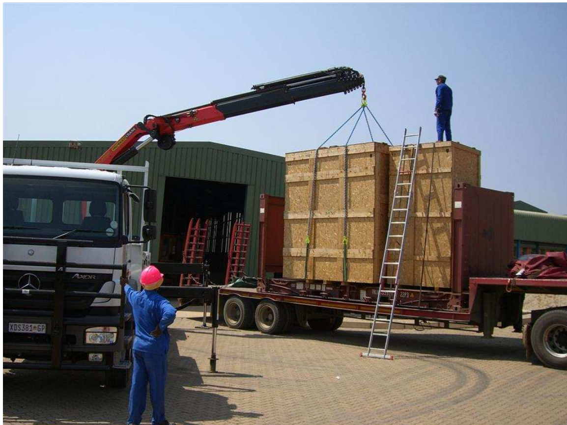
First Try- Telescope Mount crate, estimated at 3.5 tonnes.... Nope, too heavy, too far.
