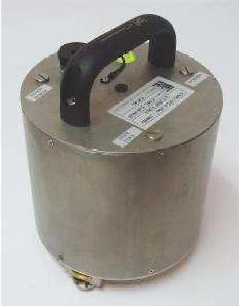
Guralp Systems CMG 40T Broadband Seismometer 60s to 100Hz
