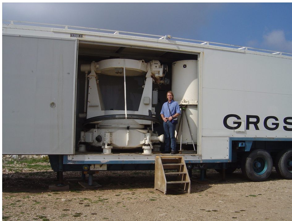
Figure 10. The one metre OCA telescope is an az-el mounted, Cassegrain telescope, which weighs about seven tons. It is too large to fit into a standard shipping container and the mount and tube will have to be specially crated and sealed against the harsh conditions to be encountered while at sea.
