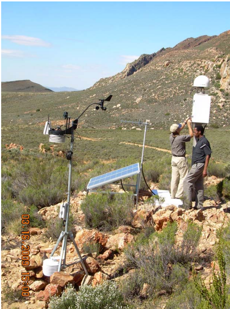
Photo 5: Existing Automatic Weather Station and GPS Antenna at the proposed site of the Matjiesfontein Observatory. The GPS Antenna position is 33^{\circ} 16' 00.9309''\text{S} , 20^{\circ} 34' 47.0883''\text{E}
