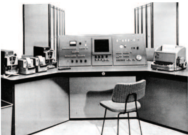
Control Console of the transistor-based version of the Stantec Zebra. © Copyright 1994 - 2006 A.J. Flavell & Glasgow University. A brochure with the specifications of Stantec Zebra can be found here .
